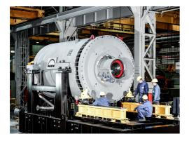
The radial compressor has a length of approximately 4 and a diameter of approximately 3 metres. *Source: MAN Energy Solutions AG*
