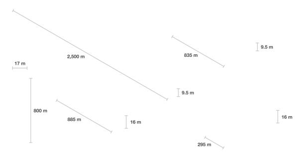
Five possibilities for realising the storage volume of 177,000 m<sup>3</sup> with tunnels and shafts. For the sake of clarity, the ratio of diameter to length is not true to scale. *Source: Philipp Roos / Andreas Haselbacher*
