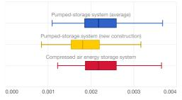
Greenhouse gas potential and damage to ecosystems from stored and re-fed electricity (Swiss supply mix) for CAES systems and pumped-storage systems (new construction or Swiss average). Damage to ecosystems is estimated on the basis of the impact of land use on biodiversity and the emission of pollutants. The ranges shown represent uncertainties and potential location-specific differences and show the median, the lower quartile and the upper quartile.
