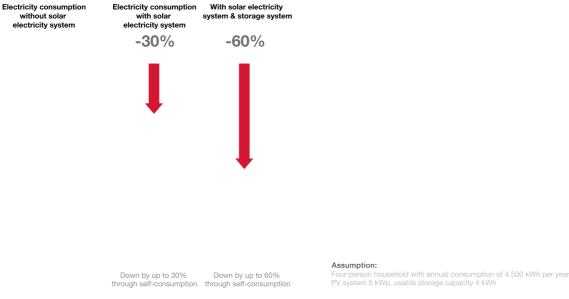
Small solar power storage units: up to 60 % less electricity from the grid.Source:
