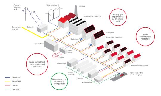
Energy hub, a multi-energy system, that is comprised of various transformation, storage and network components. It has a local steering mechanism and can be put into operation to cover different spacial scales. *Source: SCCER FEEB&D, Portia Murray*
