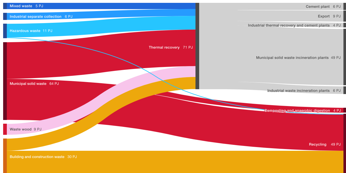
Energy flow analysis of the Swiss waste management system (2012). Source: Melanie Haupt, ETH Zürich
