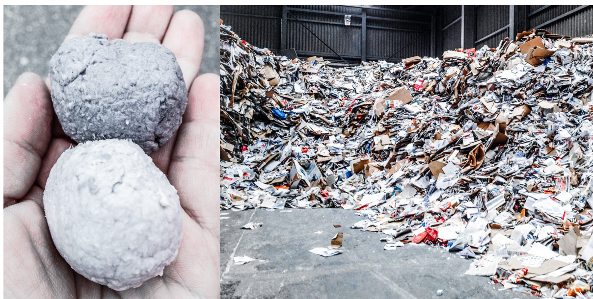
Left: fibre from paper recycling before and after deinking. Right: storage facility with mixed waste paper and cardboard at the former Utzenstorf AG paper factory. Source: Melanie Haupt, ETH Zürich
