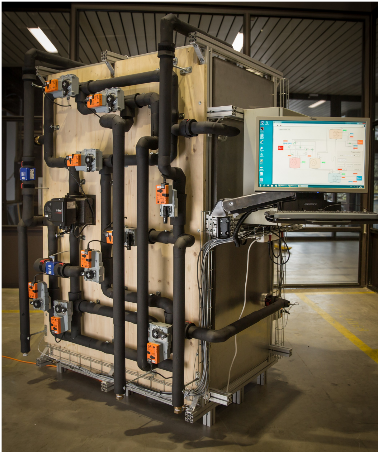
The newly developed adsorption heat pump: in the future, such plants should use waste heat for heating and cooling.
