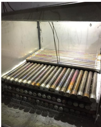
Steel pipes for latent heat storage contain a special substance mixture. Viola Becattini
