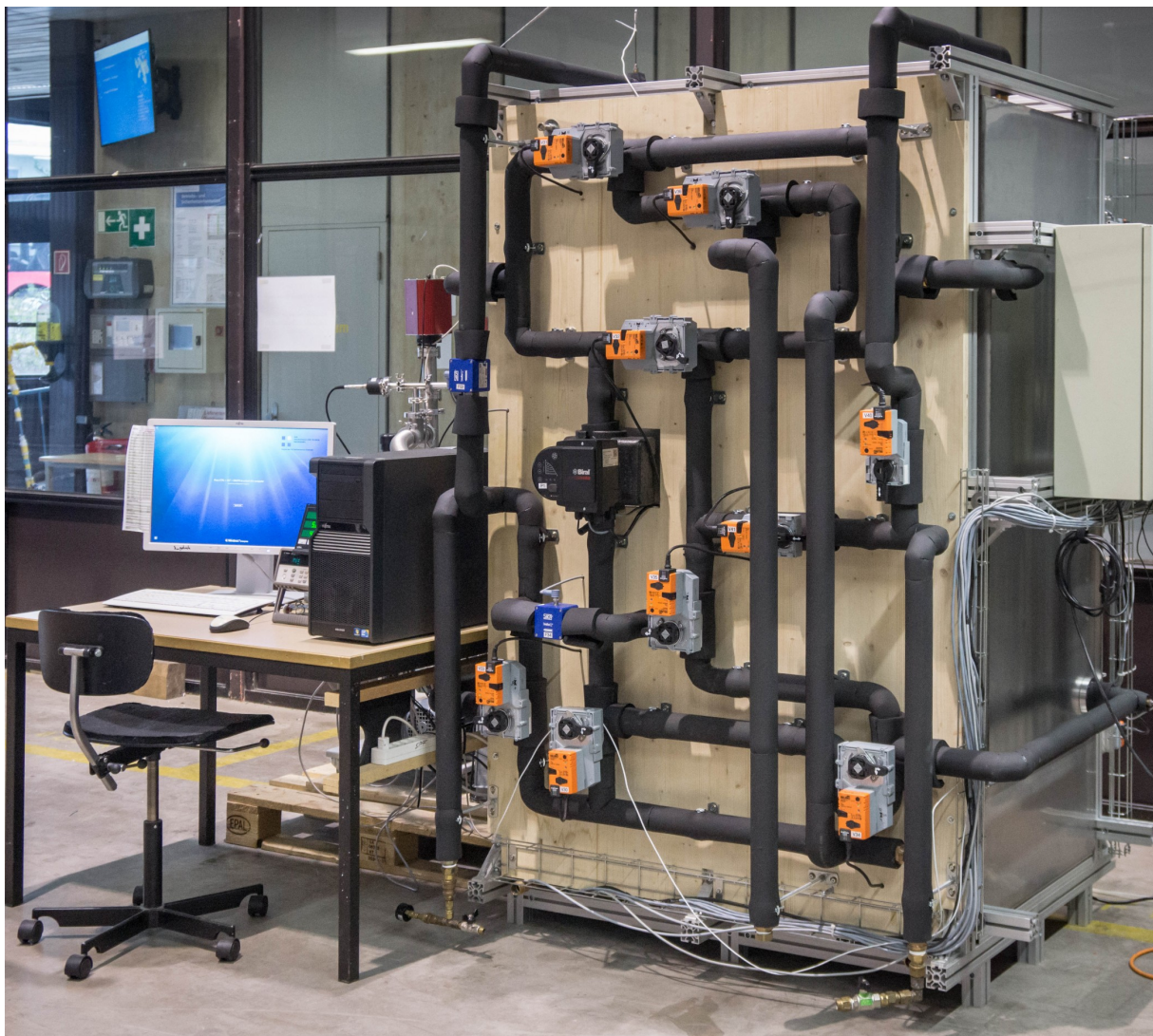
The prototype of the newly developed adsorption heat pump. Such systems could in future use waste heat from factories, for example. Source: Institut für Solartechnik
