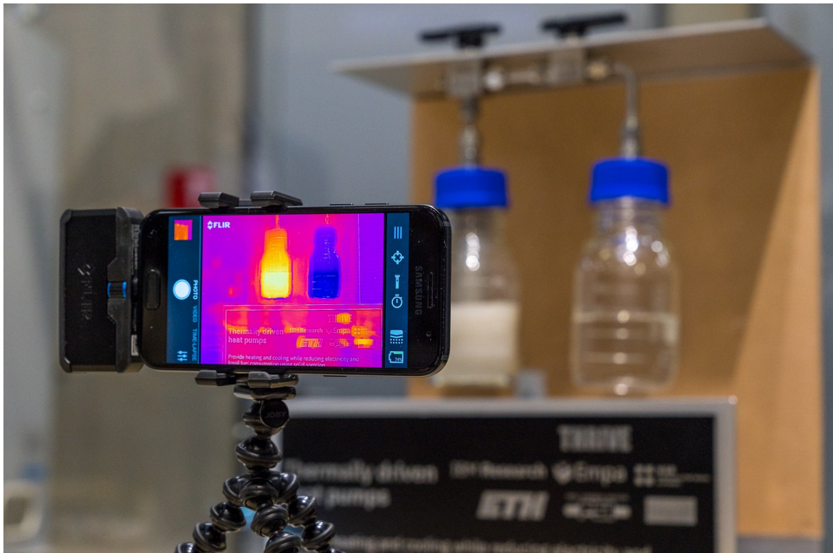
Visible heat: an infrared camera shows the temperature differences during an adsorption process. Institut für Solartechnik, HSR
