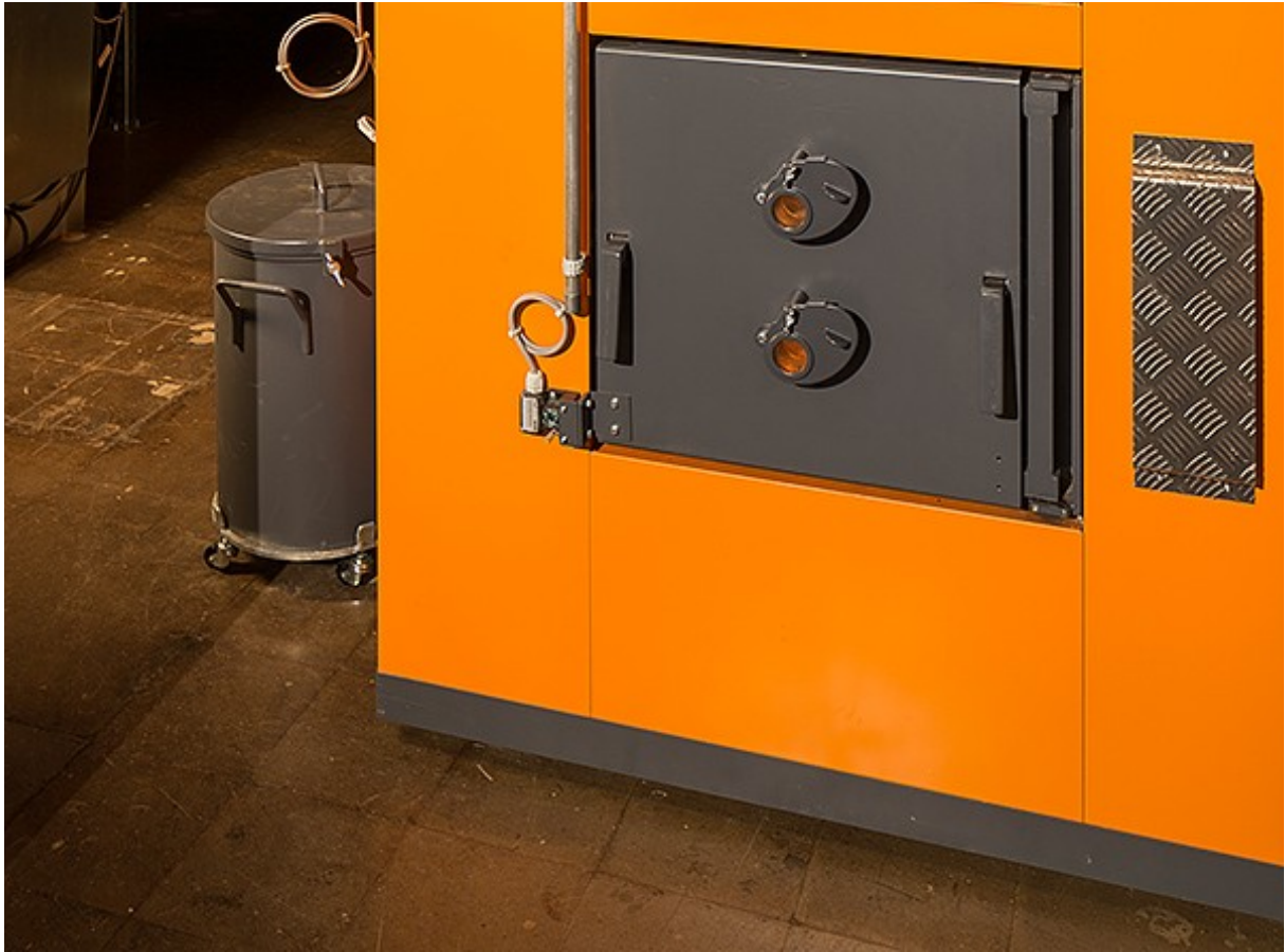
With automatic combustion systems, energy can be generated from wood without the air being heavily polluted. Source: Schmid AG energy solutions
