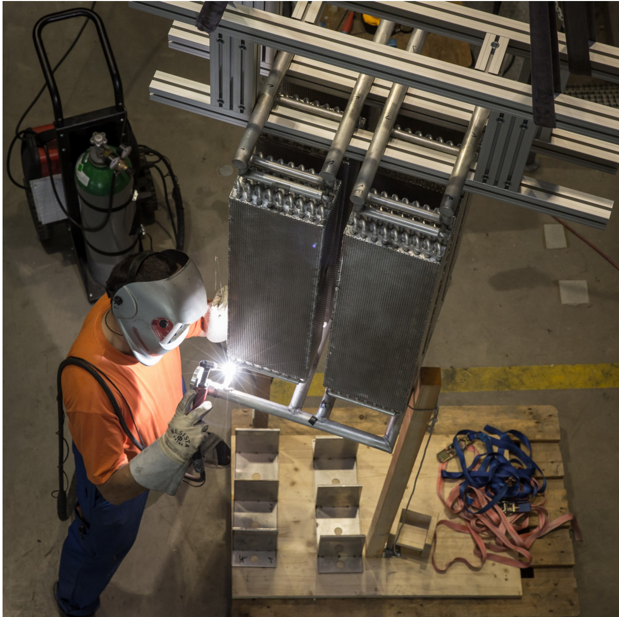
The new heat pump takes shape: Walter Camenisch from the University of Applied Sciences Rapperswil welds the heat exchanger elements together. SPF, HSR
