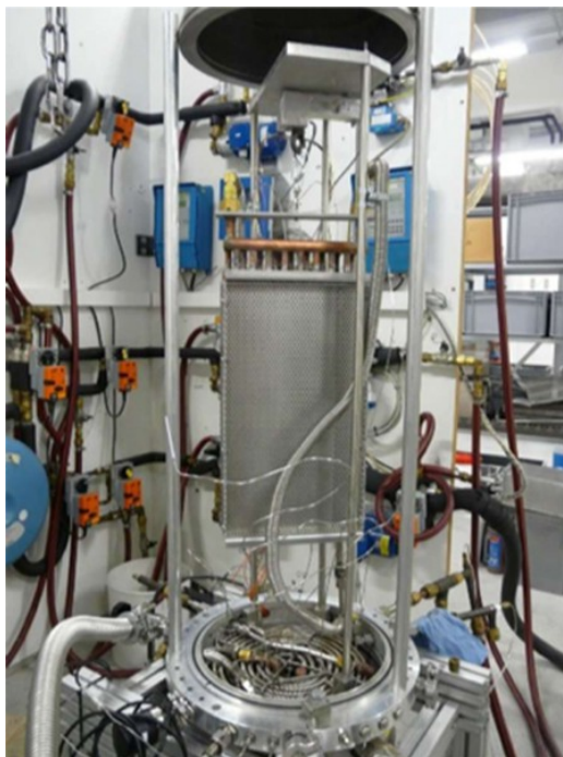
The measuring chamber is open in the photo: from the round refrigerant reservoir at the bottom, the steam enters the heat exchanger where it is adsorbed and compressed. At the top, a balance beam measures how much steam is stored in the heat exchanger. SPF, HSR
