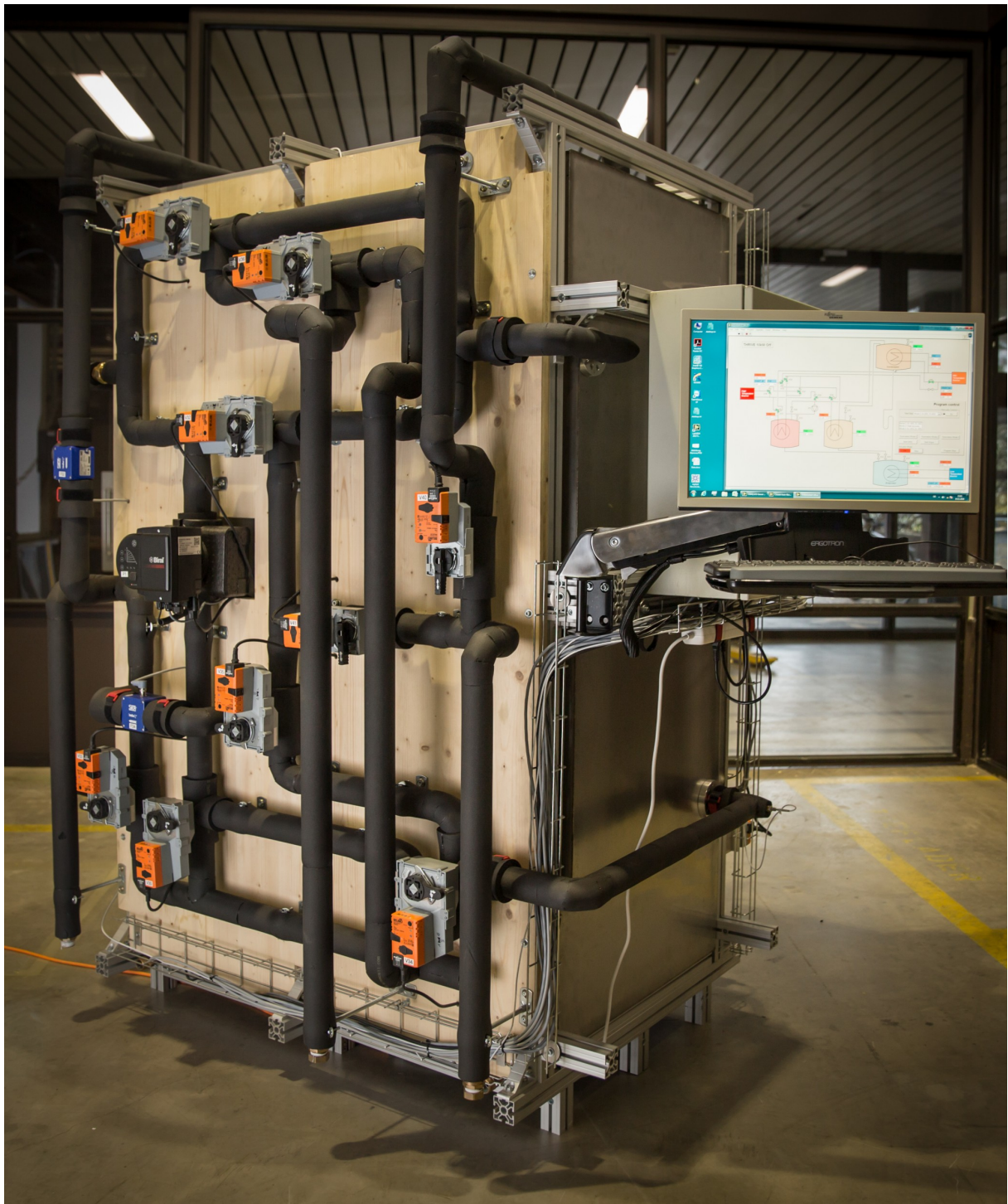
The newly developed adsorption heat pump: in the future, such plants should use waste heat for heating and cooling. Source: Institute for Solar Technology, University of Applied Sciences Rapperswil (HSR)
