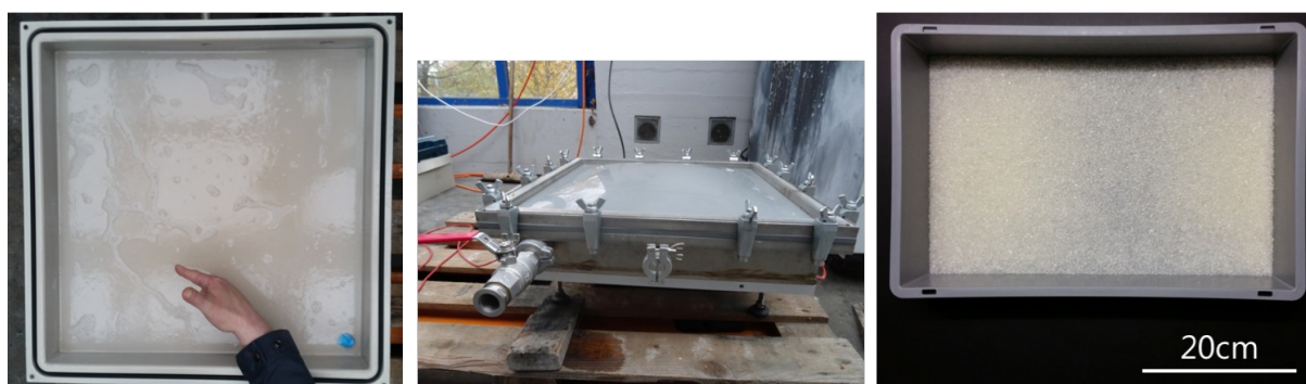
The production of the improved silica gel: from the suspension (left) through to the drying process and the product itself, the silica beads. Empa
