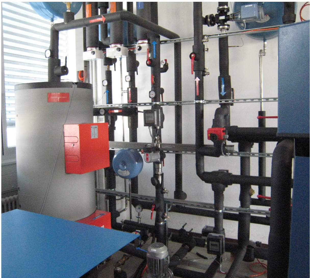
For experiments in the laboratory: the thermohydraulic system simulates the functioning of an adsorption heat pump. Source: HEIG-VD
