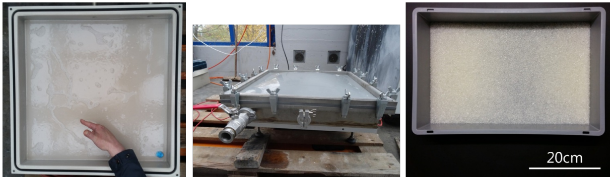
The production of the improved silica gel: from the suspension (left) through to the drying process and the product itself, the silica beads. Empa
