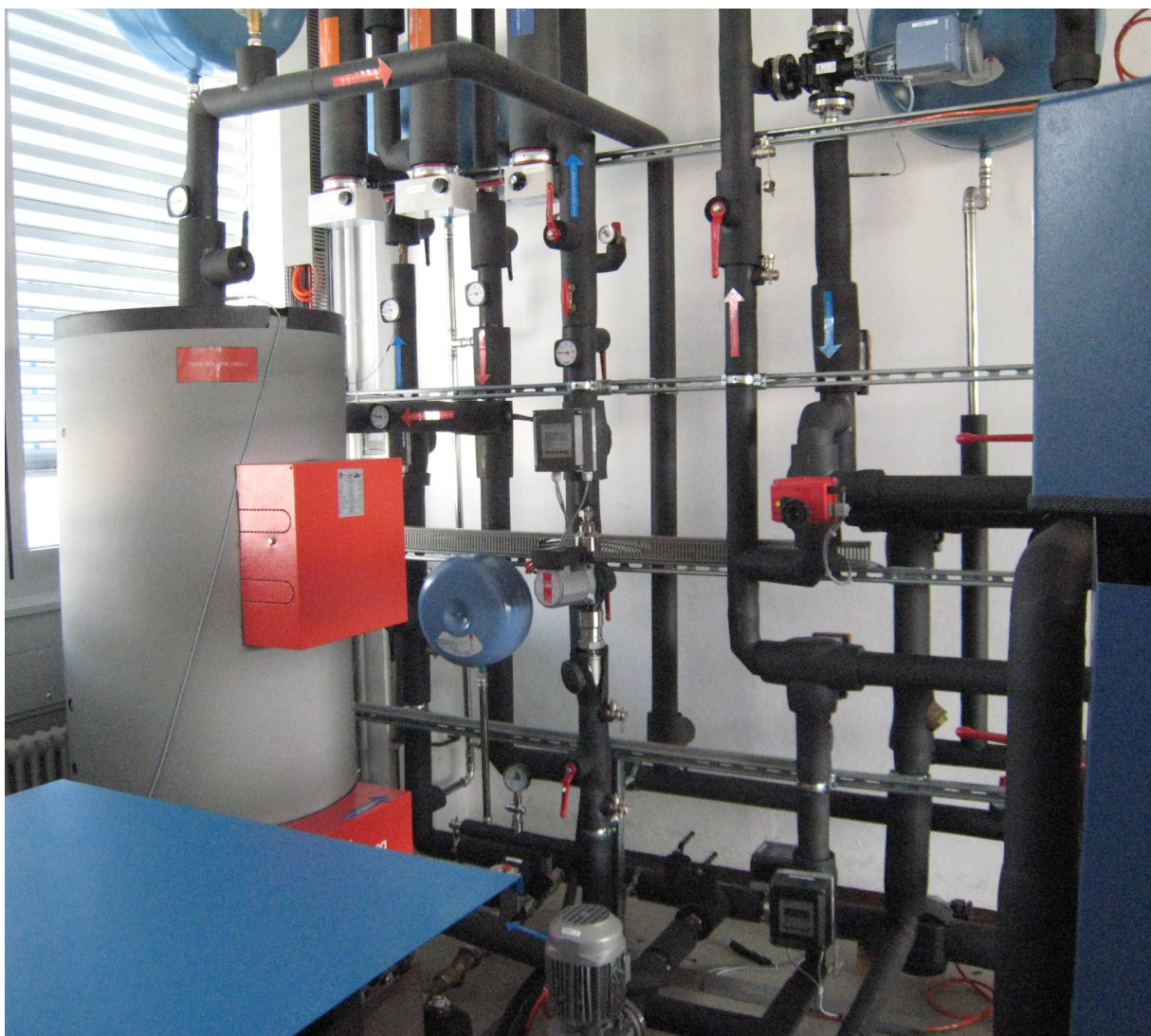
For experiments in the laboratory: the thermohydraulic system simulates the functioning of an adsorption heat pump.
