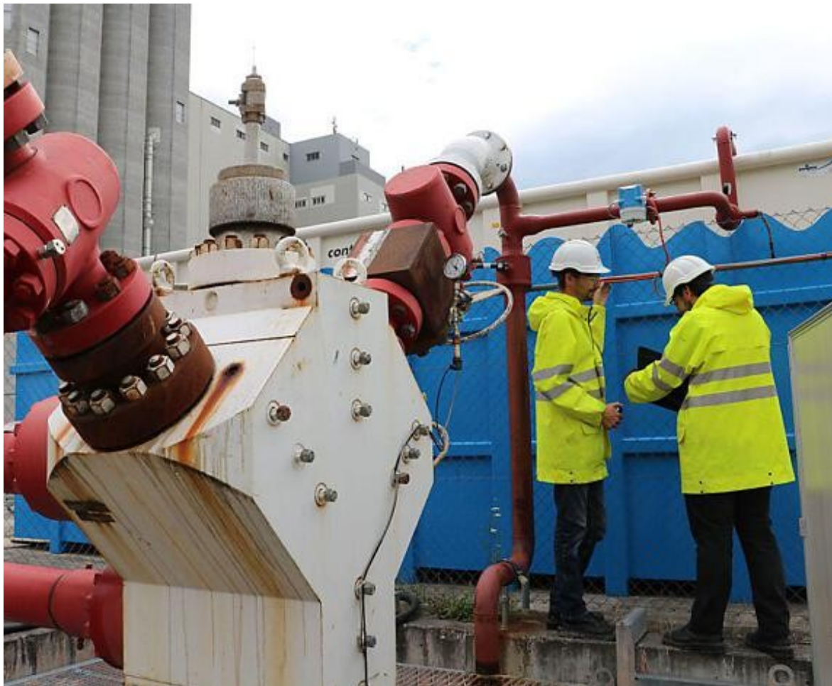
The borehole remains unused for the time being – the Basel pilot project for the geothermal generation of electricity and heat was discontinued due to earthquakes. Source: IWB/Erik Rummer
