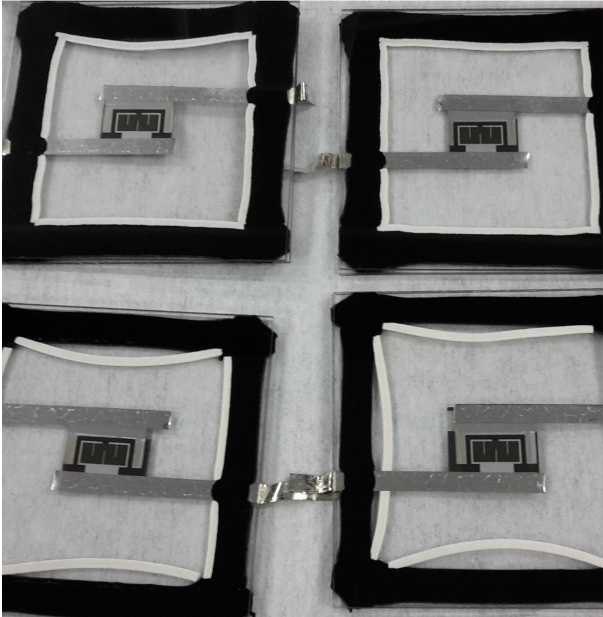
Upscaling from a laboratory scale to extensive solar modules is one of the remaining hurdles standing between perovskite solar cells and their industrial mass production. *Source: Final Report*
