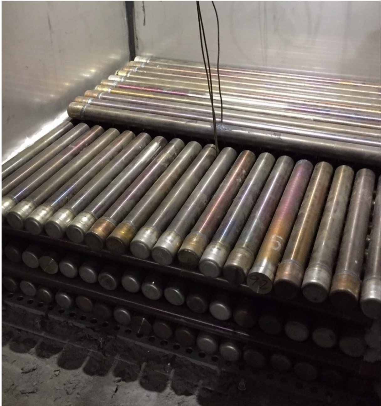
Thanks to this latent heat storage system, heat can be captured and electricity stored more efficiently. Source: Viola Becattini
