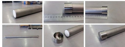
In the laboratory: a steel tube containing the phase change material. Sophia Haussener
