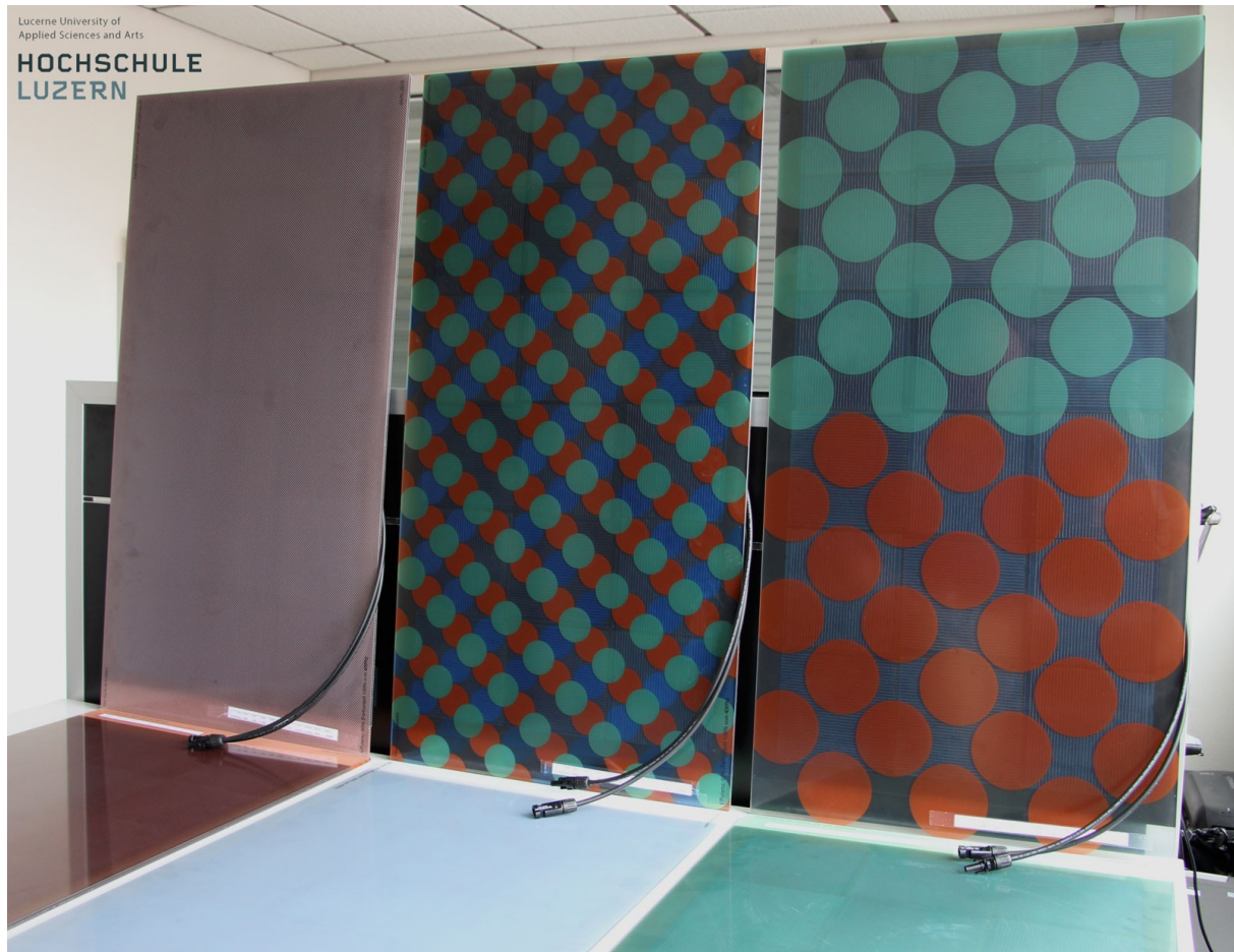
Patterns printed on PV modules. Stephen Wittkopf
