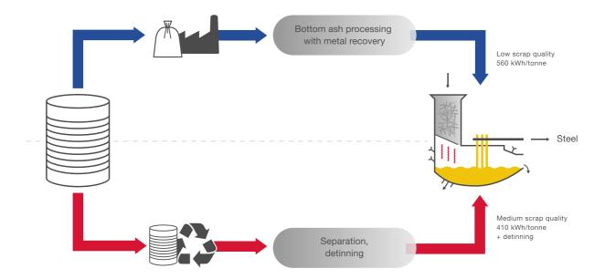
The influence of quality for tinplate recycling. While separate collection results in average scrap grades, the scrap from MSWI plants (without subsequent processing) is of a low quality. This has a major impact on electricity consumption in the recycling sector. Source: Melanie Haupt, ETH Zürich (basierend auf Haupt et al. (2017),
