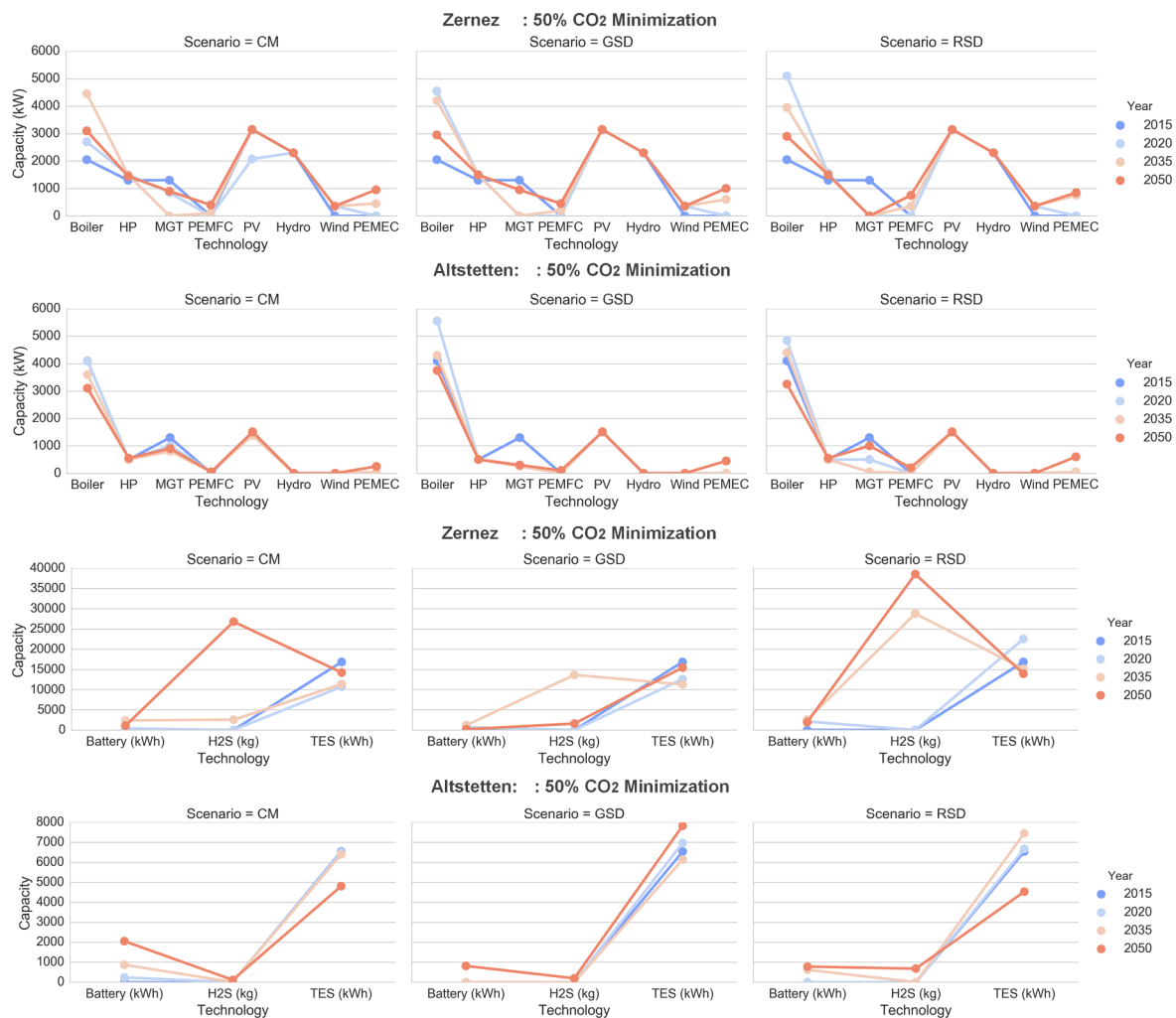
Fig. 9. Conversion (above) and Storage (below) technology sizing for the 50% CO 2 minimization objectives.
